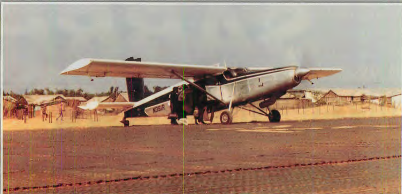
An Air America Swiss-made Pilatus Porter PT6 STOL aircraft, was an eight-seat, high wing monoplane of all-metal construction that could land on a dime. Photo: Nat Helms
