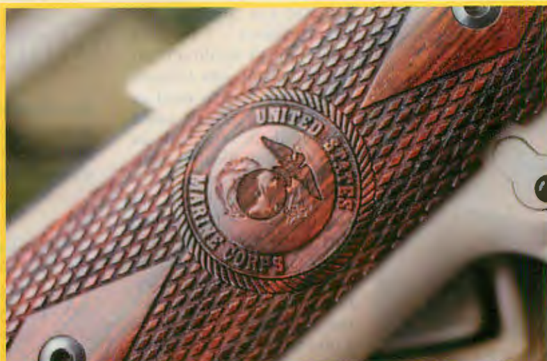
The USMC logo appears on both large diamond checkered walnut grip panels of that pistol and is laser engraved.
